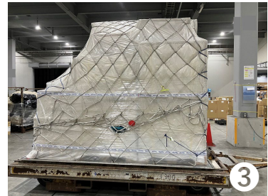
Cargoes must be shrink-wrapped for waterproof. Then, ULD and cargo must be tightly fixed by cargo rubber-net not to move.
